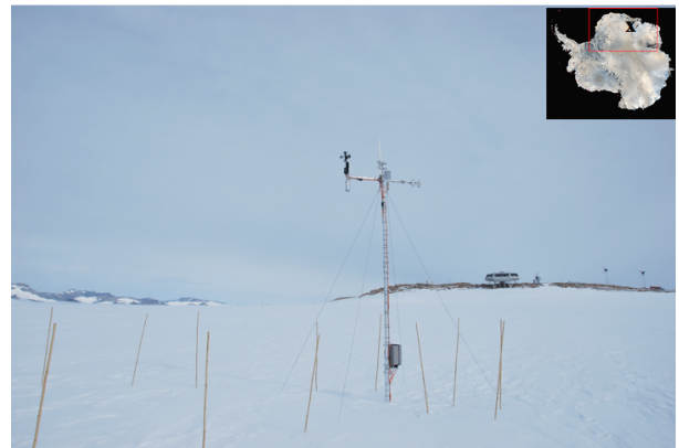
Figure 1. Automatic Weather Station installed as part of the HYDRANT project near the Belgian Antarctic station Princess Elisabeth (photo - February 2010). The AWS is designed by the IMAU group ( www.projects.science.uu.nl/iceclimate/aws/ ).
